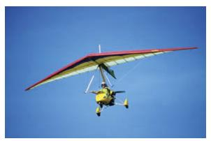
The "trike" is a large, engine-powered hang glider, with a fuselage (includi landing gear) suspended from the wing. Instead of launching into the air fr side of a hill, as traditional hang gliders do, the trike is able to self-launch f level surface by rolling on its wheels and using the power of its rear-mount engine.
