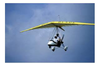
A pilot can also shutdown the engine and soar the trike if the rising therma sufficiently strong. However, the lift-to-drag ratio and sink rate of a heavy t not as conducive to soaring as a traditional hang glider. To stay aloft, a typ trike needs rising air of about 450 feet per minute. Lift-to-drag ratio commo varies from a low of 7:1 to a high of 10:1.
